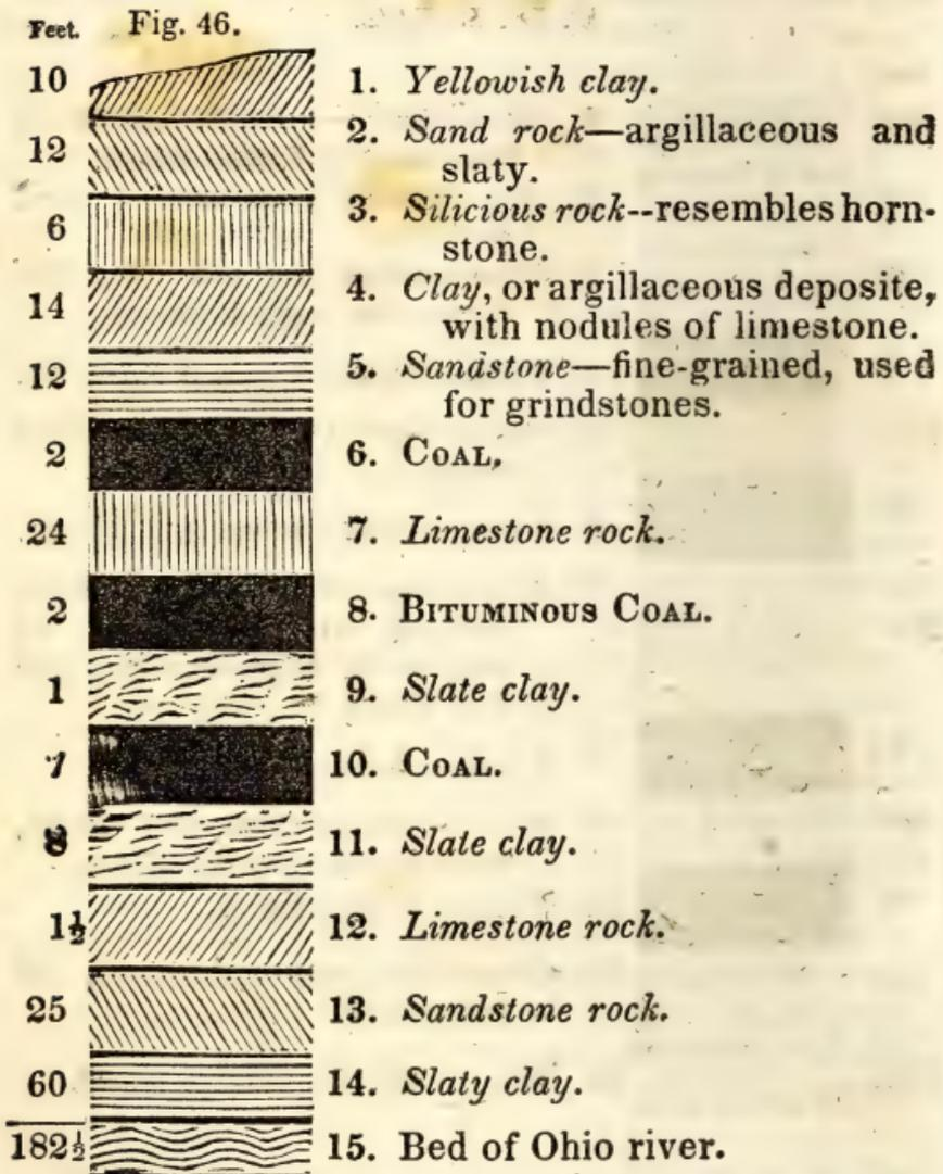
NOTE.—A mile and a half from this section, a bed of coal 12 feet thick crops out from the side of a hill at such an angle of elevation, that, were it continued, it would be at the height of 200 feet above stratum No. 1 of the series !
